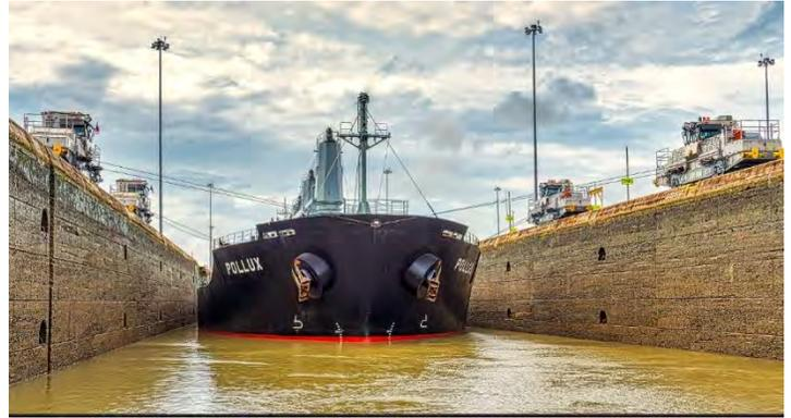
*These are the third generation of electric locomotives on the canal. The track is 5' gauge with a rack in the middle and power conduit on the land side. The locomotives do not pull vessels through the locks. The ship provides its own propulsion. The "mules" act more as a brake and to keep the vessel in the center of the lock. The vessel is under the control of the canal pilot during the transit. While known as mules, animal traction was never used in the Panama Canal.*
